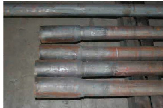
Upset ends forging for shank, so that threads can be made
