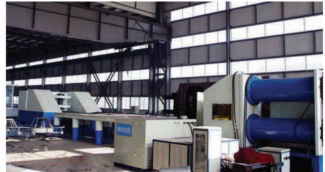
Breaking load testing of the whole tie rod system
