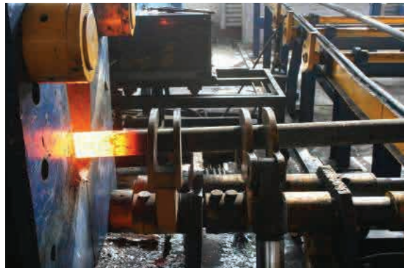
Upset ends forging for shank, so that threads can be made
