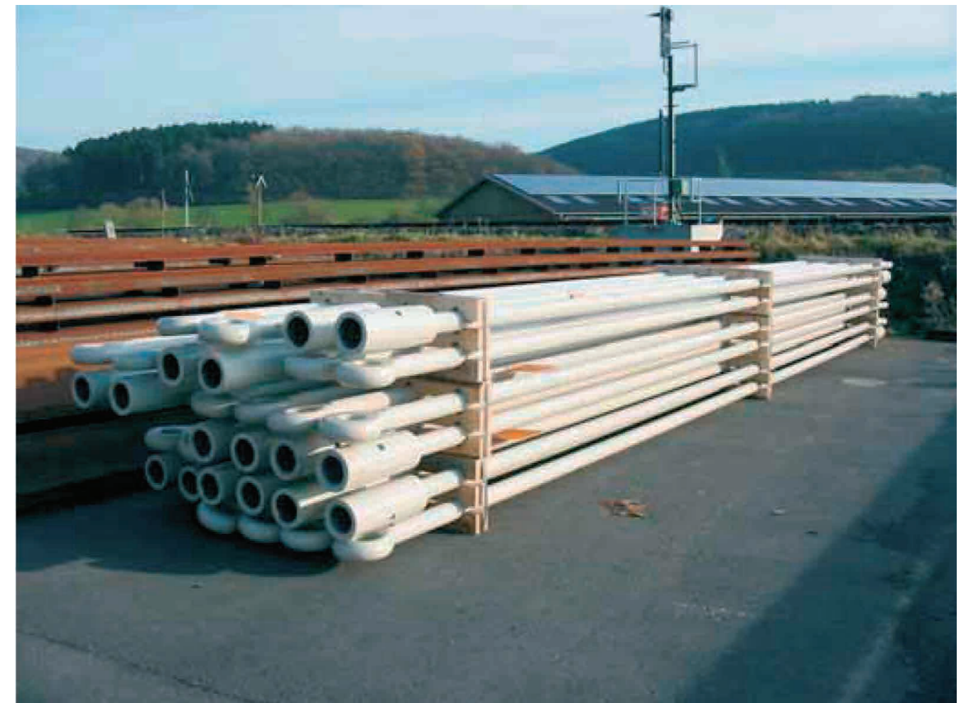
Epoxy paint coating
